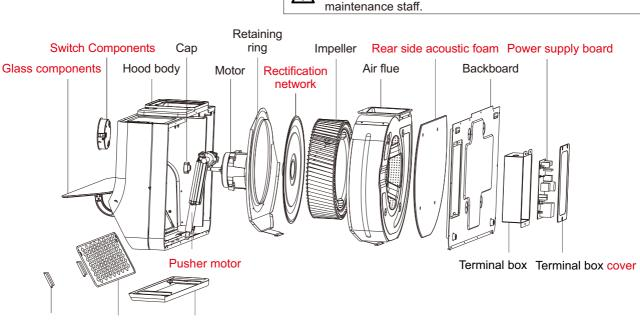
LED Lamp Filter mesh Oil cup
