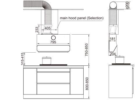
c. Installation method when the hanging cabinet width is 435-800mm (the following installation method takes 450mm as an example)
