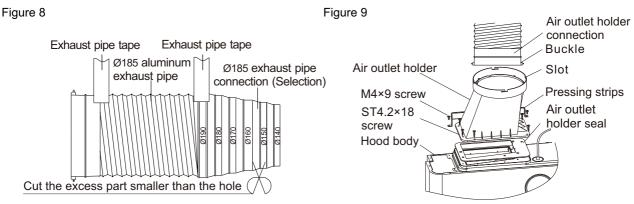
Note: During installation, straighten the aluminum exhaust pipe to avoid noises in semi-stretched state.Excess part may be cut with a wire cutter.
